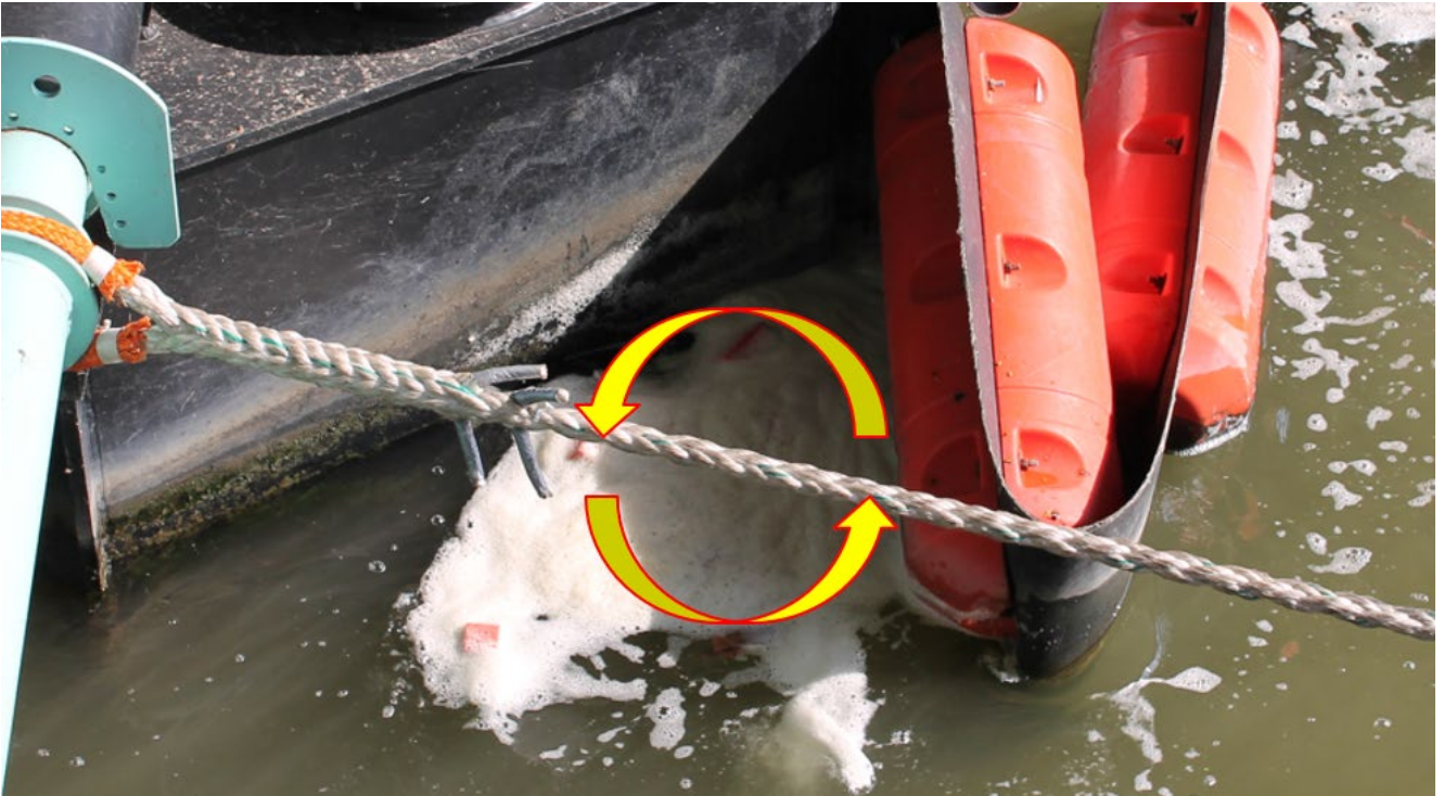
Figure 12: Circular flow behind booms
