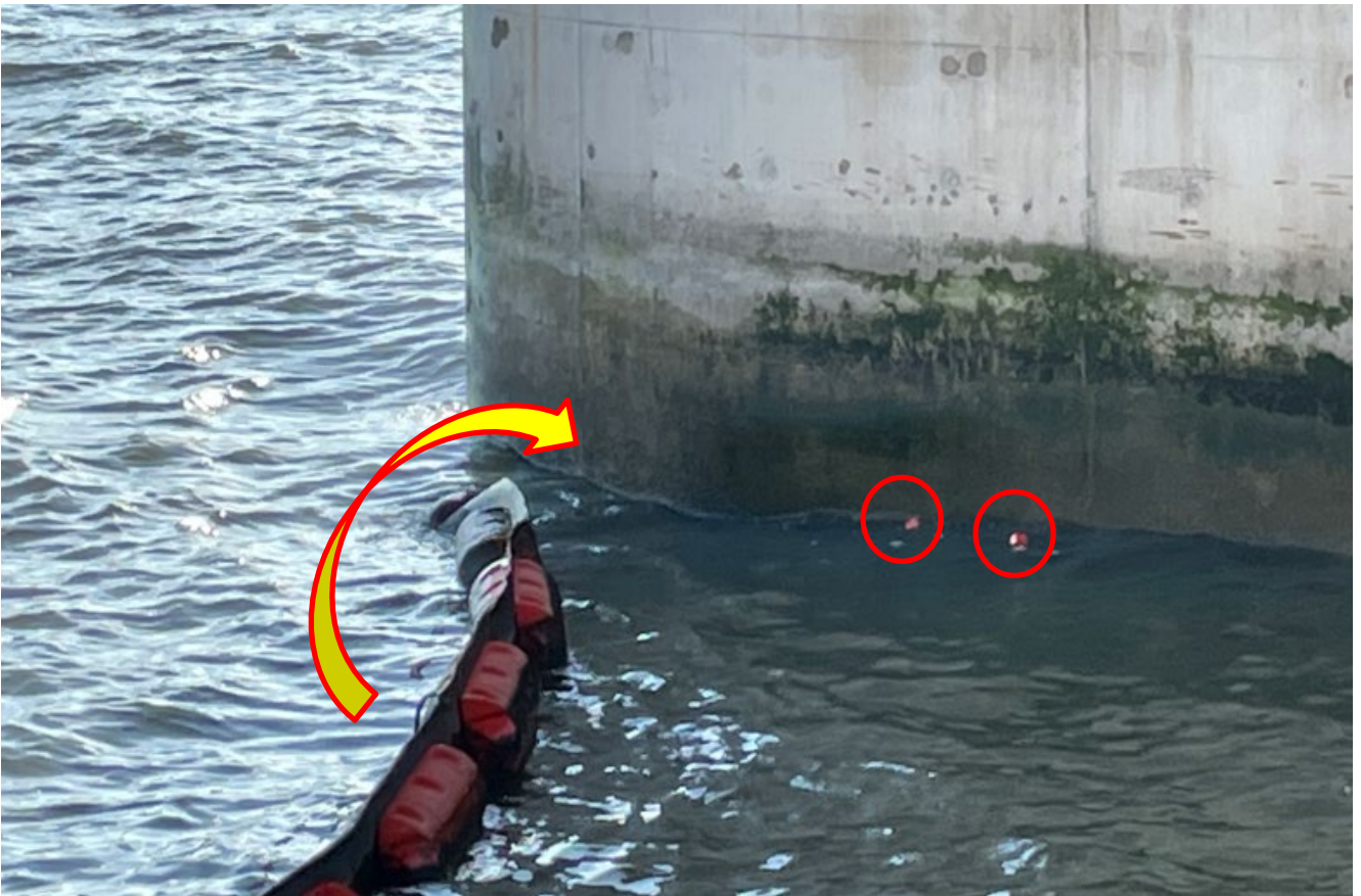
Figure 13: Tracers between bridge pillar and boom
