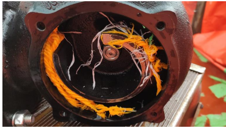
Figure 3-20: The pump jammed on the yellow 5mm rope
