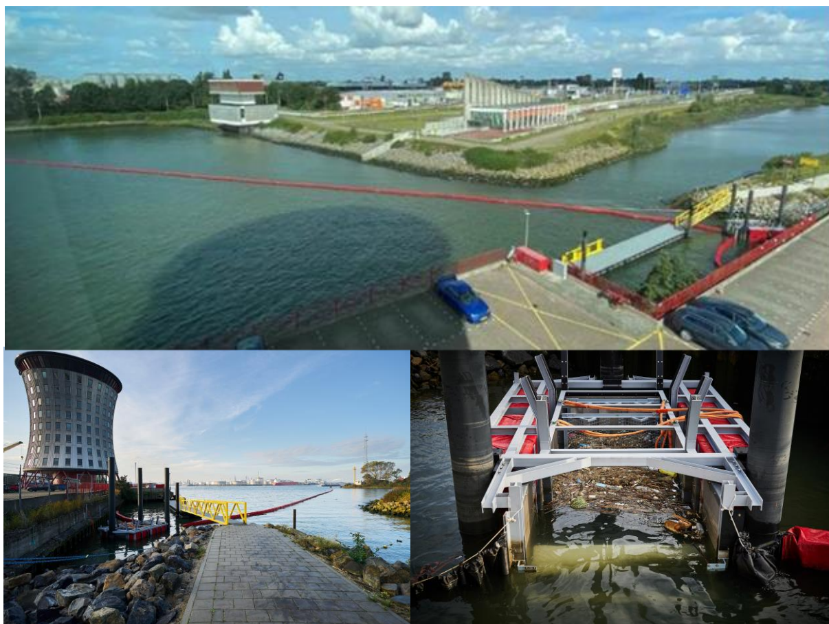
Figure 10 Overview of the Catchy collection deployed at the Vijfsluizerhaven (top), wide view of the location (left) and filled cage (right).
