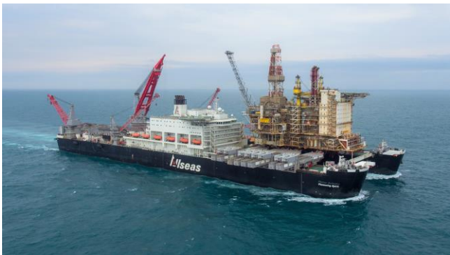
Pioneering Spirit with a decommissioned topsides (left) and jacket (right), heading for a dismantling yard
