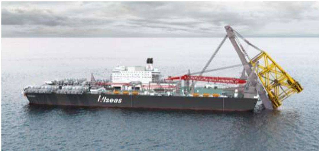
Impression of how the Gyda jacket ready for transport in a near-vertical position
