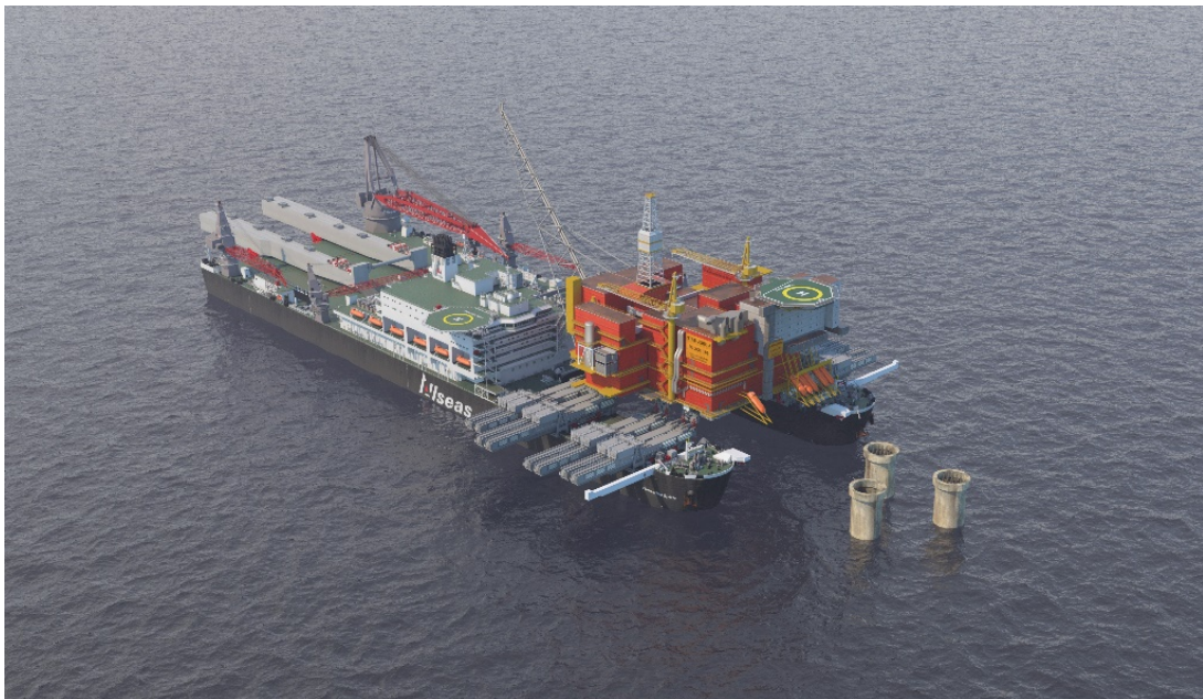
Animation still of Pioneering Spirit removing the Statfjord A platform topsides (available by request)
