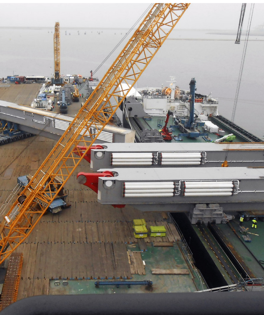
CLAMP OPTION: In operation the beams are joined in pairs, supporting a single connector which can be either a clamp, as above, or a yoke.
