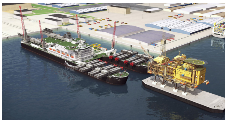
INSHORE TRANSFER: In normal service, the 200-metre long Iron Lady will be used for handover of topsides to or from Pioneering Spirit .
