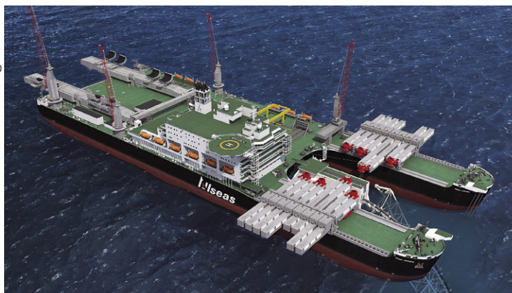
DUAL-PURPOSE: Pioneering Spirit's elaborate stinger system will be hung off in the bow slot when the vessel performs a pipelay contract.
