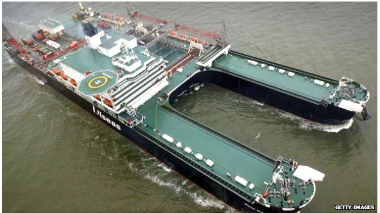
The specialist Pioneering Spirit is the world's largest platform decommissioning vessel
