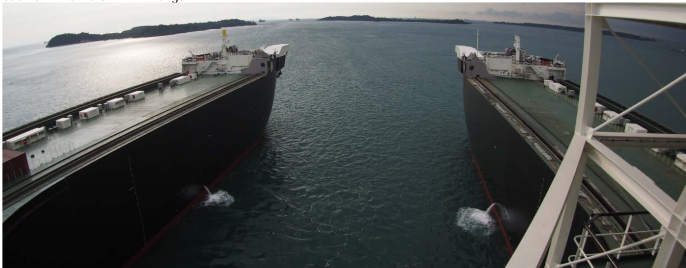
The slot in the bow is having a length of 122 mtr and width of 59 mtr
