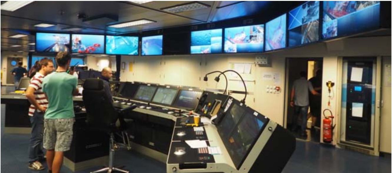
Top seen the forwards navigation bridge equipped with the latest state of the art equipment including an LR DP (AAA), fully redundant Kongsberg K-Pos DP-22 and 2 x cJoy system
