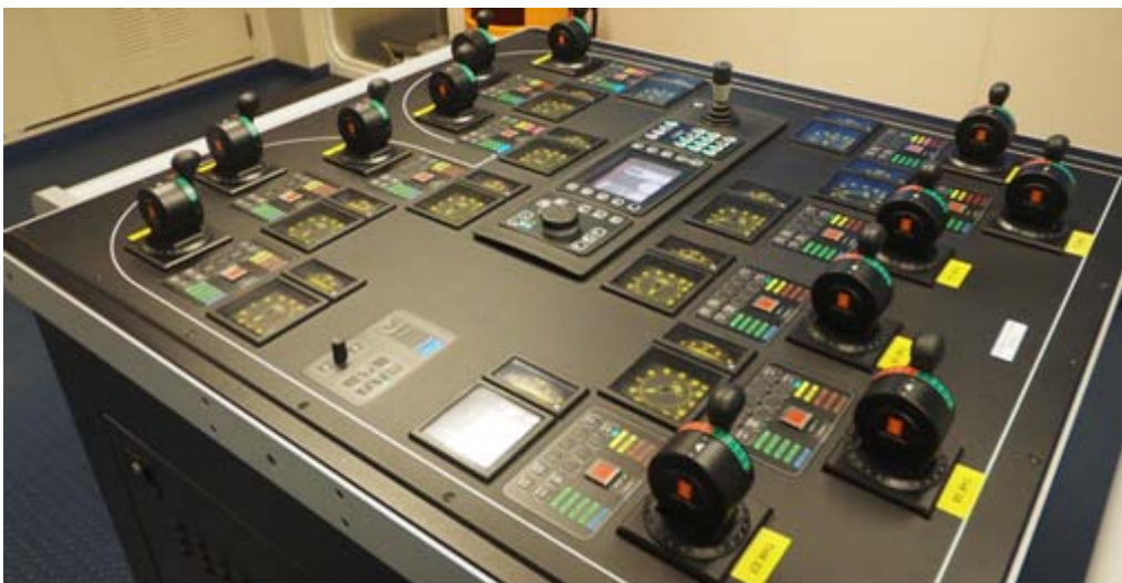
Top seen the forwards navigation bridge equipped with the latest state of the art equipment including an LR DP (AAA), fully redundant Kongsberg K-Pos DP-22 and 2 x cJoy system
