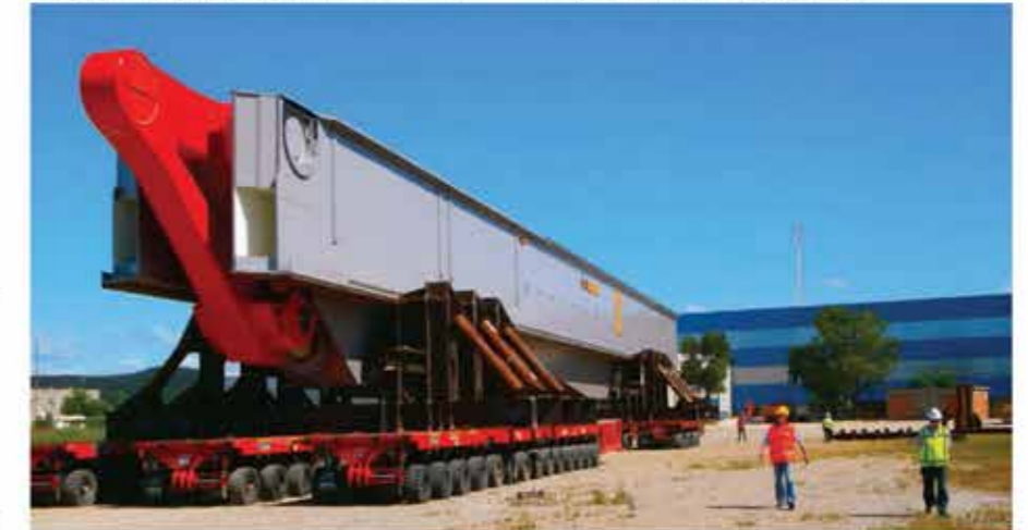
Load out of the topsides lift system beam number one. Photos from Allseas.
